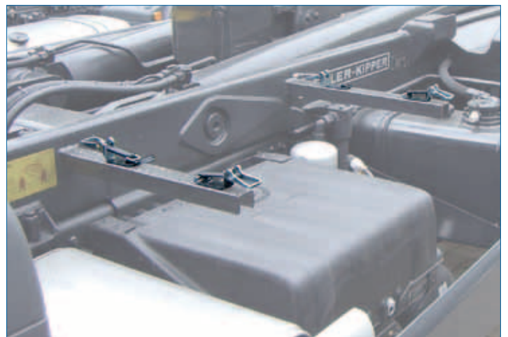
Shovel and broom brackets
