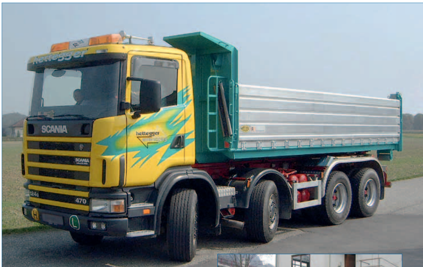
Roll-off tipper with side tipper superstructure
