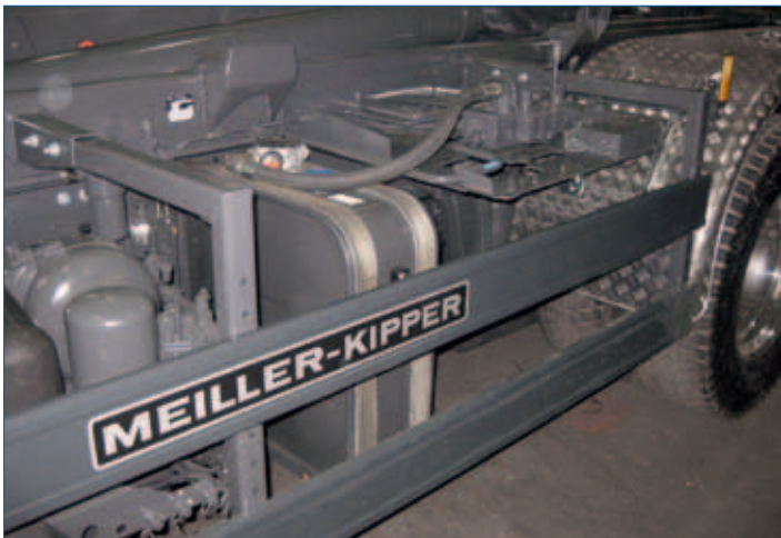
Attachment for oil tank and side safety guard
